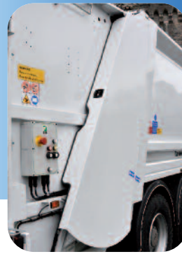
Carriage plate cylinders mounted outside the hopper area protected by external cover, easy access for maintenance from the outside of hopper area.
