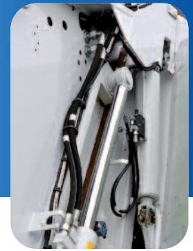
Carriage plate cylinders mounted outside the hopper area protected by external cover, easy access for maintenance from the outside of hopper area.
